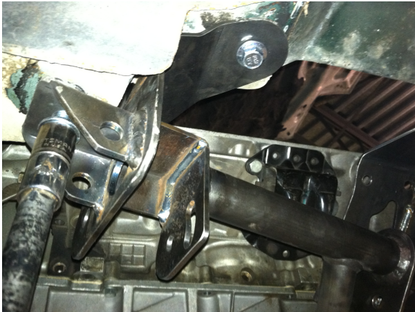
Fastening UMI k-member to chassis
