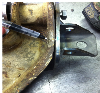
Clearance grinding on factory arm
