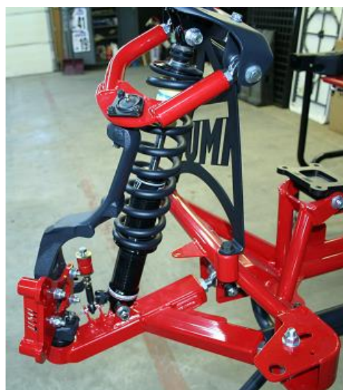
Figure 3: Installed View of Upper and Lower A-arms.
