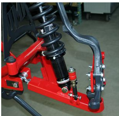
Figure 2: Driver Side Arm Installed.
