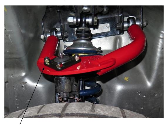
Only tighten ball joint nuts when the arm is attached to the mount in the wheel well.
