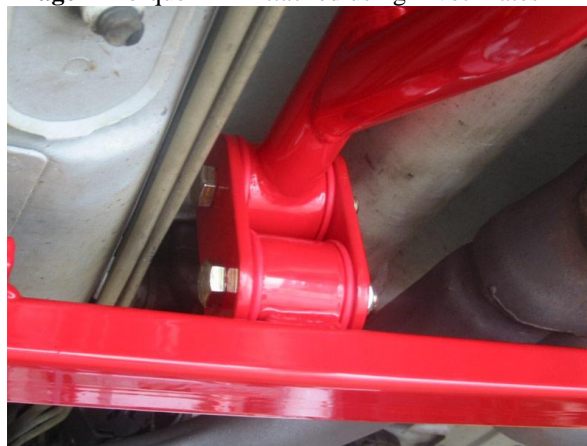
Image 2- Torque Arm Attached using Pivot Plates
