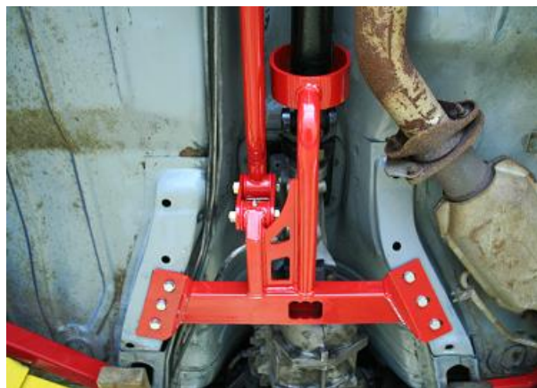
Image 3- Item # 2215 Installed with Drive Shaft Loop
