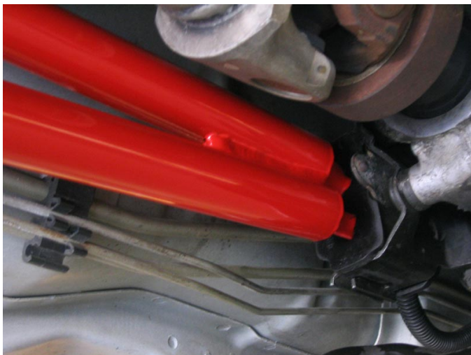
Image 3- Rear Torque Arm Mount Bolted in Place
