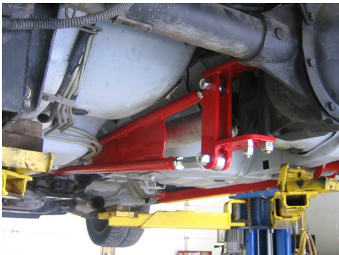
Image 3- Rear Torque Arm Mount Bolted in Place
