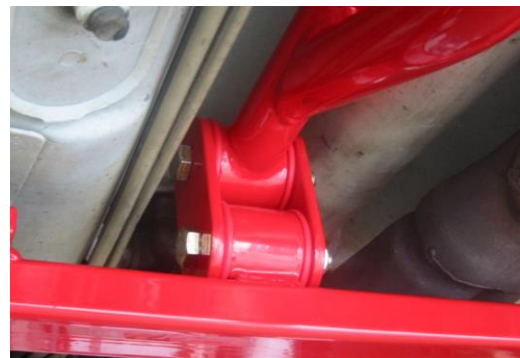
Figure 2: Torque Arm Attached using Pivot Plates
