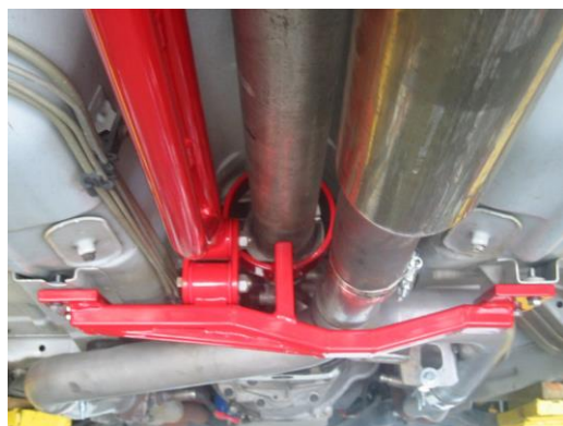
Figure 3: Item # 2203 Installed with Front Drive Shaft Loop
