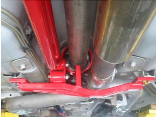
**Figure 3:** Installed with Front Drive Shaft Loop
