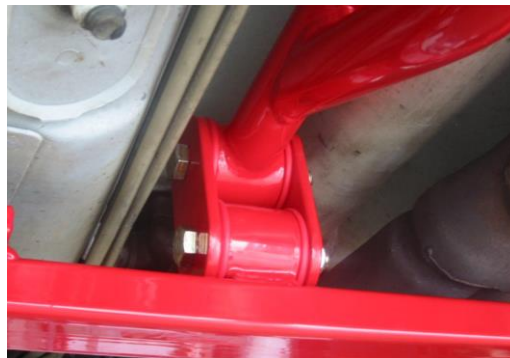
Figure 2: Torque Arm Attached using Pivot Plates
