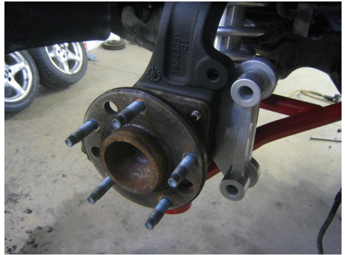
Image 2- Drivers side bracket installed with hub
