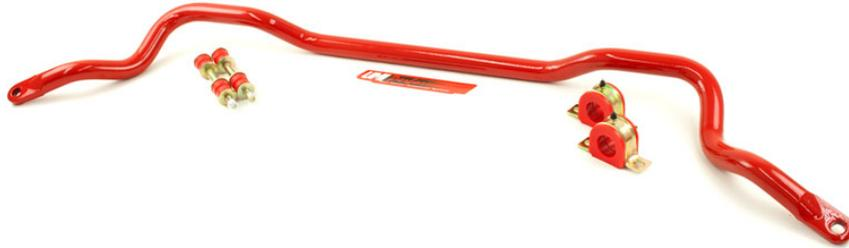
**Kit Includes-** (1) 1.375" tubular sway bar, (2) End Links and (2) sway bar bushings with clamshells
