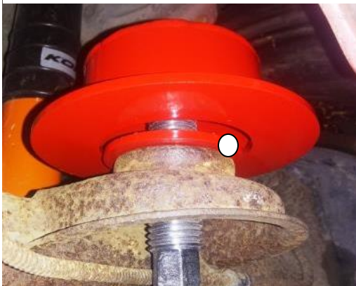
Install Passenger side, align notch toward rear of car. Notch is denoted in picture by white dot
