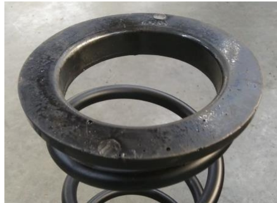
Install provided isolator on top of spring. This will go between the spring and body of car.
