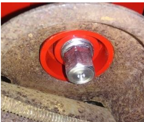
Highest recommended position of adjuster. Leave a minimum of 1 thread showing underneath the adjuster.
