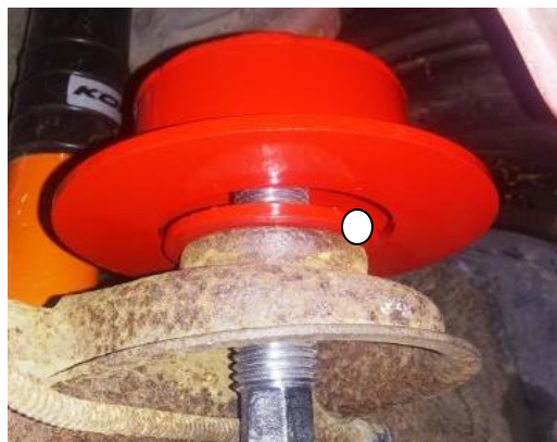
Install Passenger side, align notch toward rear of car. Notch is denoted in picture by white dot
