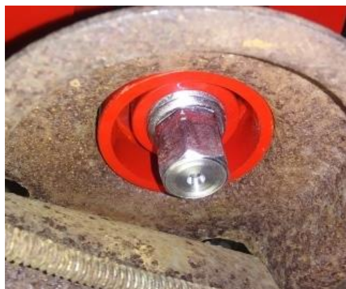
Highest recommend position of adjuster. Leave at minimum 1 thread showing underneath the adjuster.
