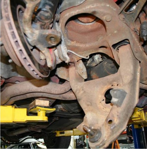
FIGURE 1: Factory spring removed.
