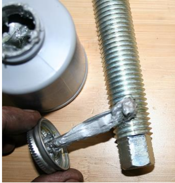
FIGURE 2: Apply extreme pressure grease or anti-seize to the threads.
