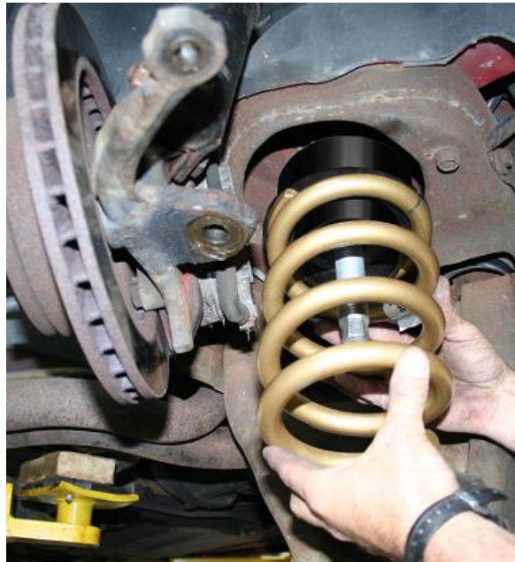
FIGURE 3: Install assembly between frame and lower A-Arm.
