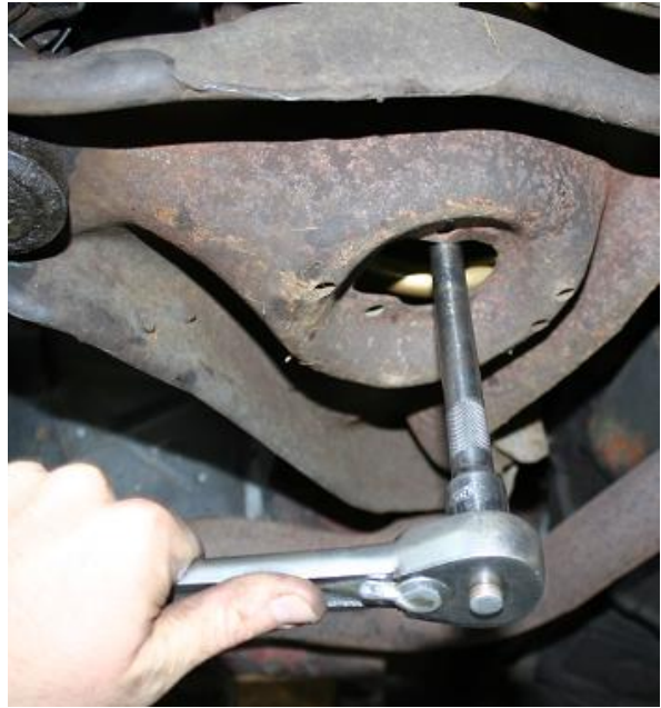
FIGURE 5: Make height adjustments with a ratchet, an extension, and a 3/4" socket. Right to raise and left to lower.
