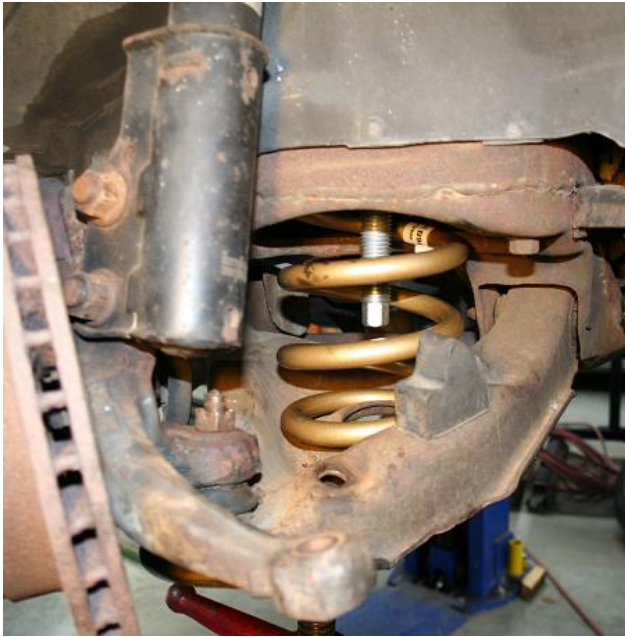
FIGURE 4: Carefully compress with jack until ball joint can be re-attached.
