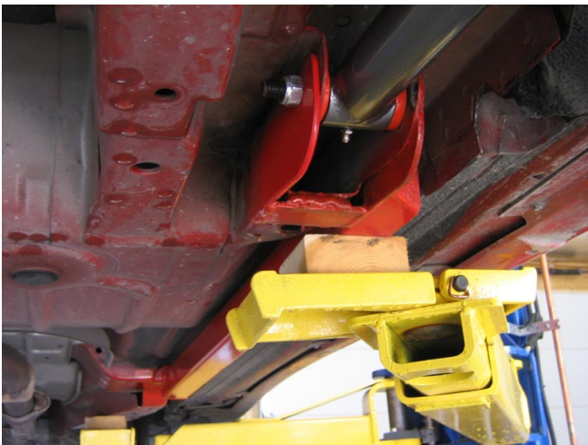
Image 3- Shows Rear Passenger Side Welded and Control Arm Reinstalled
