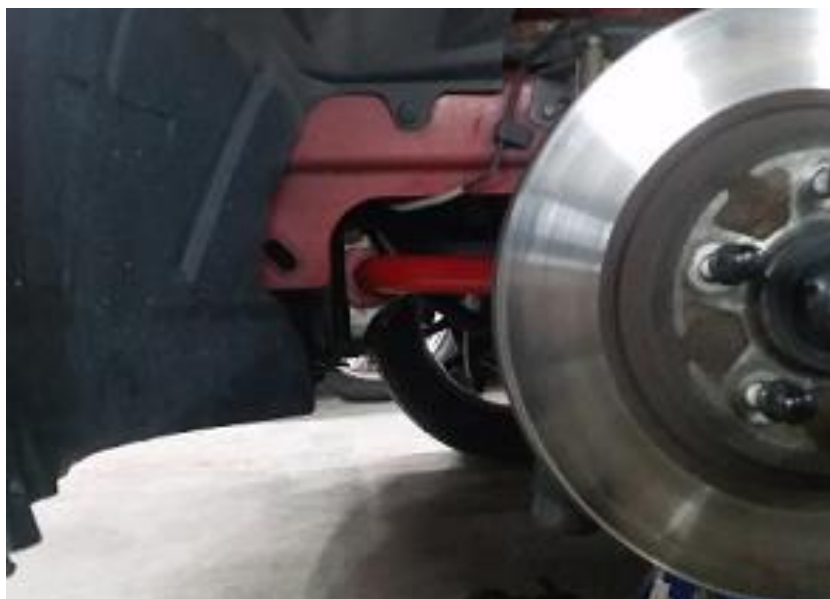
Figure 1) View of the front sway bar bracket
