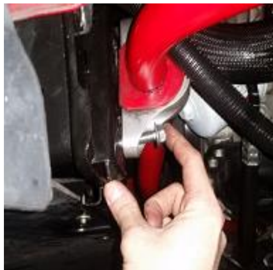
Figure 5) Aligning the plate and inserting the bolt
