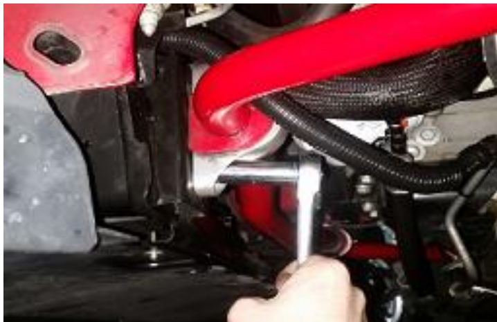
Figure 2) Removing nuts (UMI Aluminum Sway Bar Bracket)
