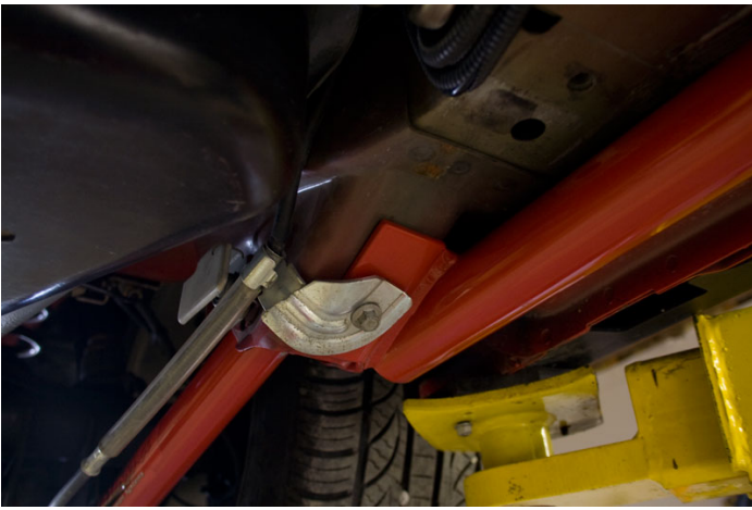
Image # 2- Drivers side fuel line cover (cut)
