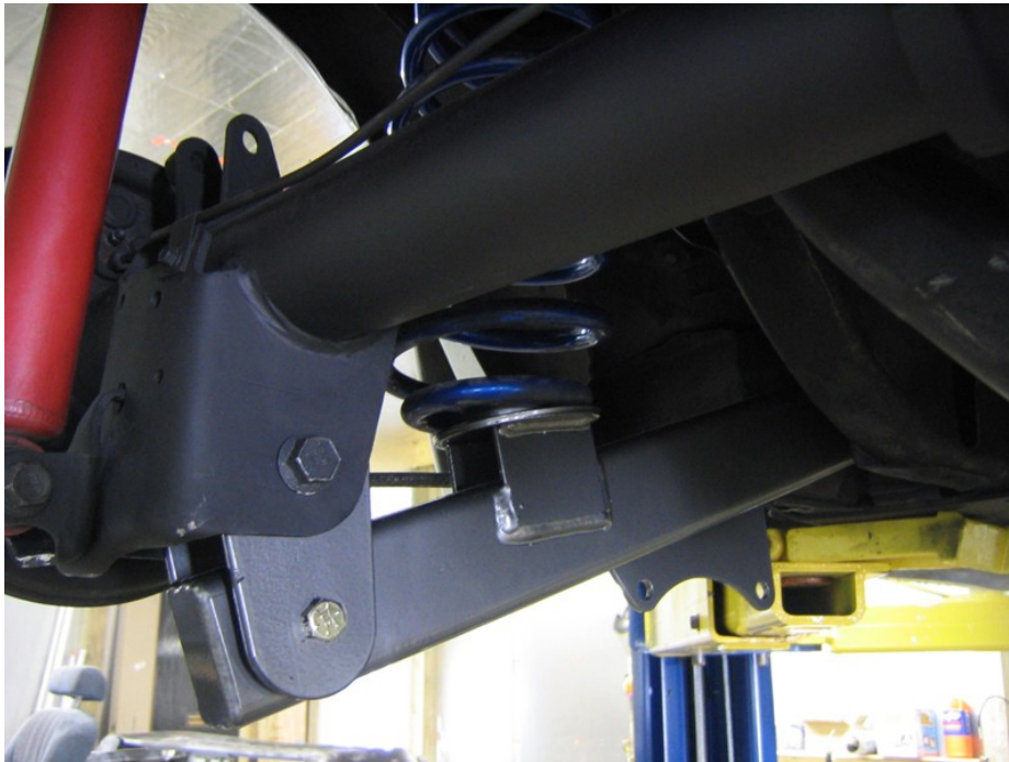
Image 1- Shows driver's side lift bar installation completed
