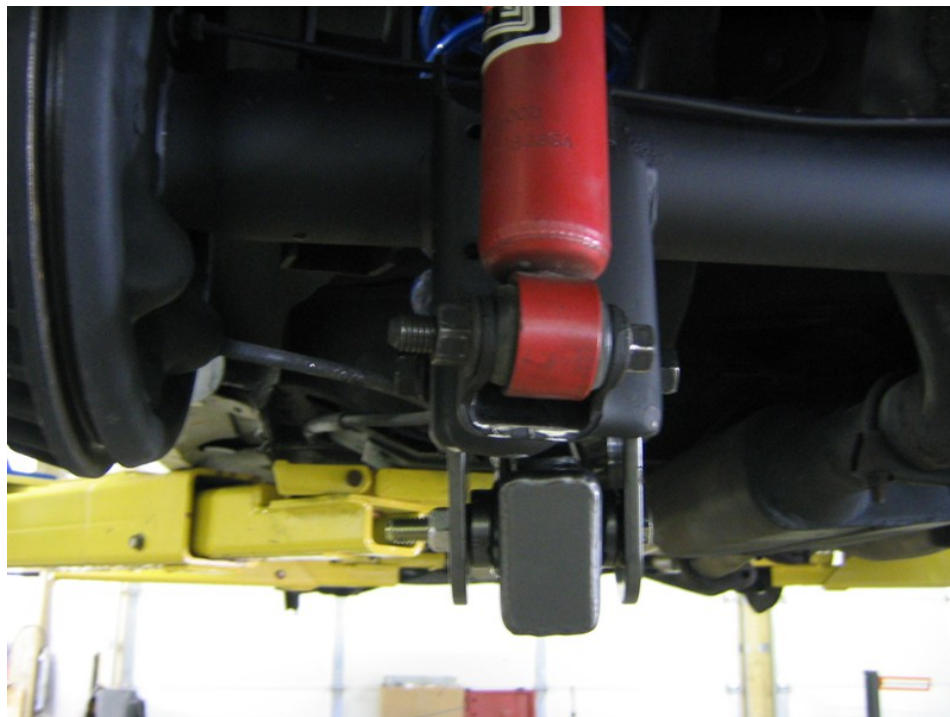
Image 2- Shows driver's side lift bar installed, picture taken from rear of vehicle.
