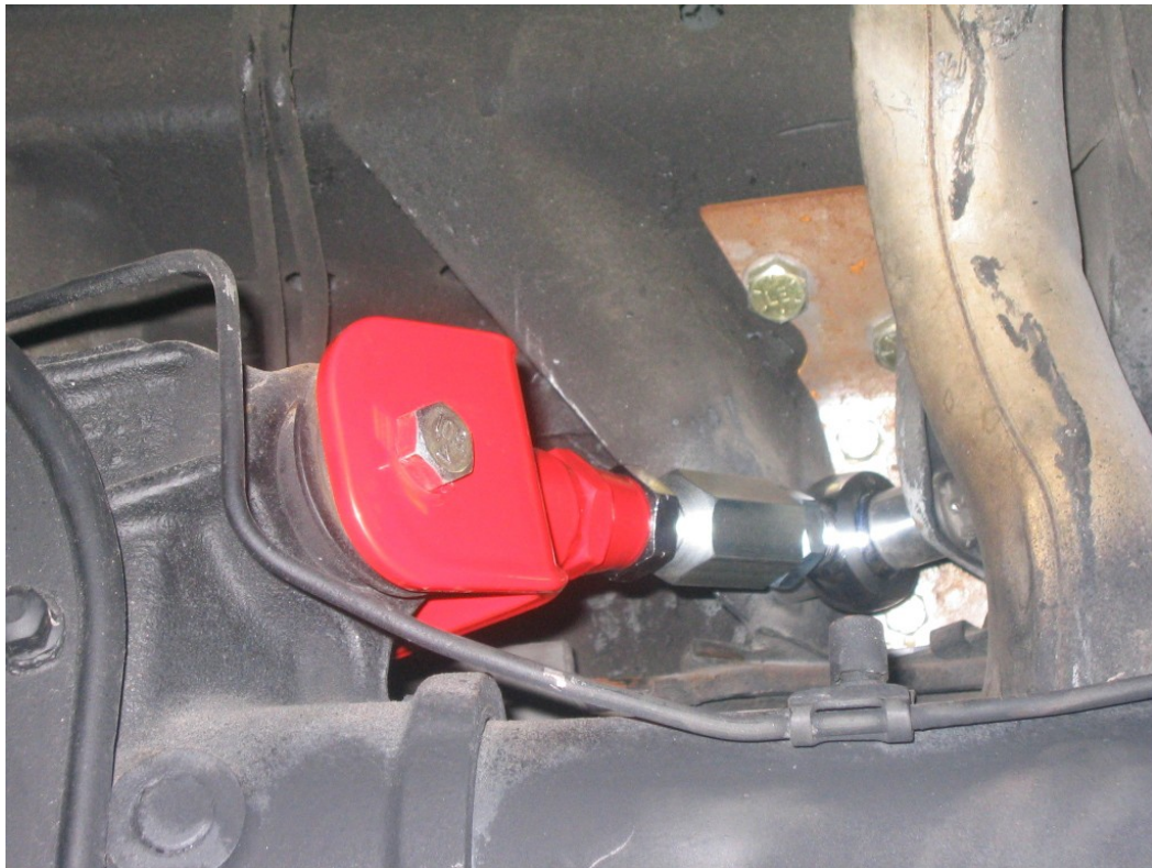
Image 2- Shows Upper and Lower reinforcement installation completed from inside the car
