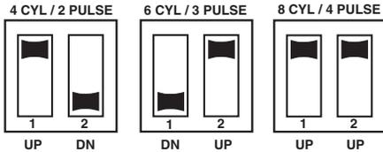
4 CYL. - Switch One up, Switch Two down.
