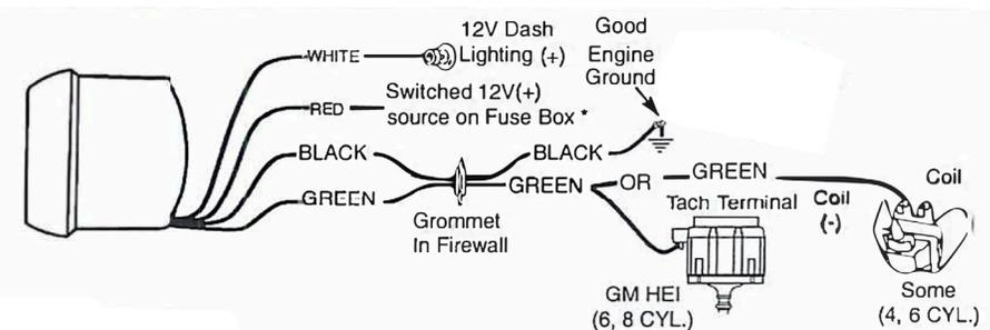
\* Optional: Wire to a switched 12V source with an in line fuse.
