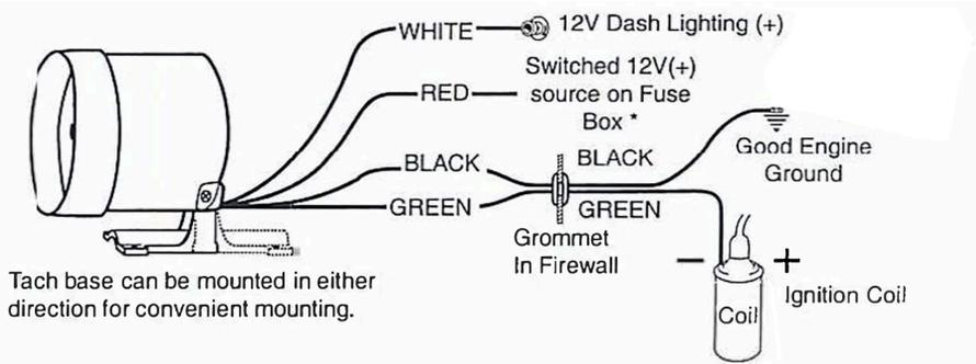
Tach base can be mounted in either direction for convenient mounting.
