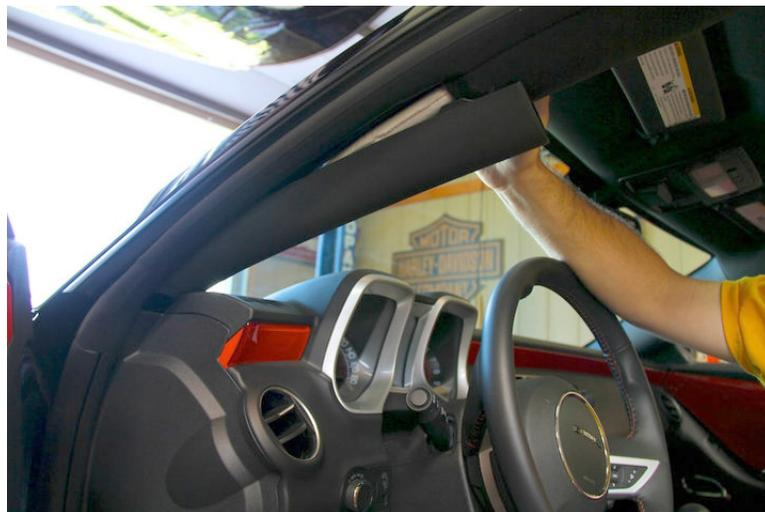
2. To start, pull the factory A pillar down. It pops out, but don't try to pull it all the way down.
