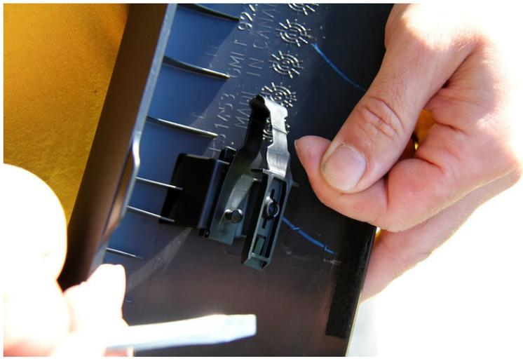
5. The safety strap is then removed from the factory pillar. The tab on the back is depressed and it slides right out.
