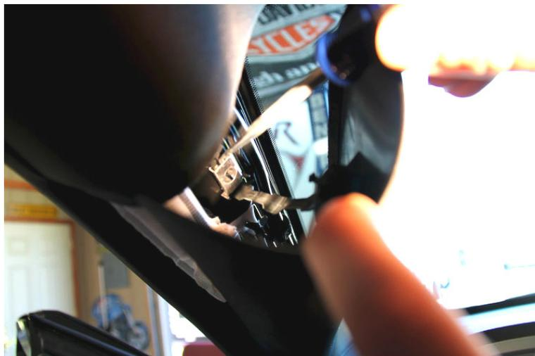
3. There is a safety strap that needs to be removed to pull the pillar away. The screwdriver is pressing into the point where it is released in this picture.
