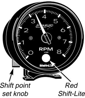
\* **Note:** If the engine is running, the shift point can't be set.
