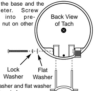
\***Note:** Lock washer and flat washer must be underhead of screw.
