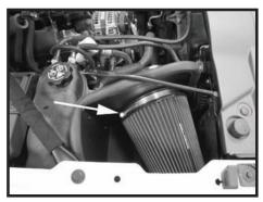
Step 13 Install the filter and fully tighten the clamp.
