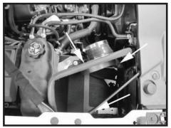
Step 10 Install the heat shield into the truck as shown by reusing the hardware from the tray. If the holes do not line up with the heat shield, see the next step to resolve this.
