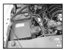
Step 5 Remove the air box assembly by pulling up and out firmly.
