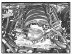
Step 16 Install the 90° boot on throttle body with the short side on the throttle body and clamp on the throttle body side to secure the boot in place. Install a second clamp but do not tighten at this time.
