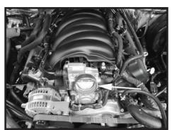
Step 15 Install the throttle body adapter ring onto the throttle body.
