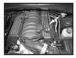
Step 2 Remove the driver side engine cover.
