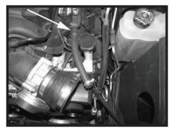
Step 12 Install the breather hose on the hose fitting on the engine.
