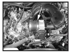
Step 15 Install the reducer coupler on the throttle body and secure the coupler in place. Install a second clamp but do not tighten at this time.
