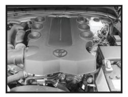
Step 2 Remove the engine cover.
