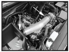
Step 16 Install the end of the intake tube into the reducer coupler on the throttle body. Install the velocity adapter in the heat shield and onto the angled coupler. Once the tube is in the desired location, tighten all the clamps.
