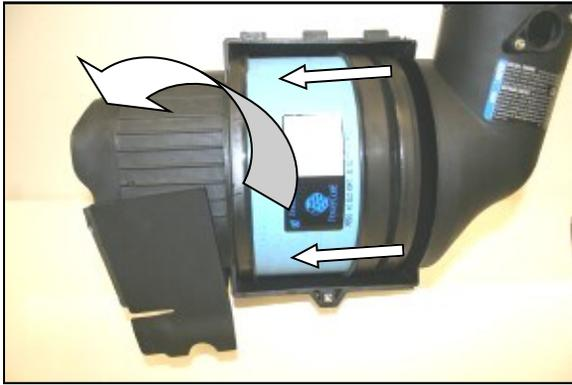
3. Slide the factory air filter away from the elbow of the airbox and remove it.
