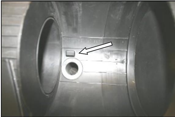
5. Locate the raised rectangle in the bottom of the factory airbox. It is important to engage the notch at the bottom of the Airaid Premium Filter to ensure proper fit and a good seal.
