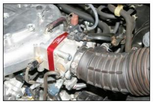
5. Reinstall the factory intake tube, and tighten the hose clamp. Reconnect the metal tube to the intake tube. Reconnect the throttlebody wiring connector. Reinstall the engine beauty cover.
