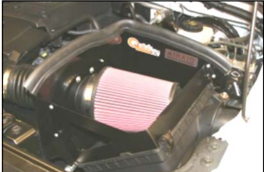
14. Install the Airaid Premium Filter (#1) on the MAF adapter and tighten the clamp. Next install the weather strip (#5) on top of the Quick Fit Panel as shown. For an easier install, start at the front of the Quick Fit Panel and work your way towards the back.
