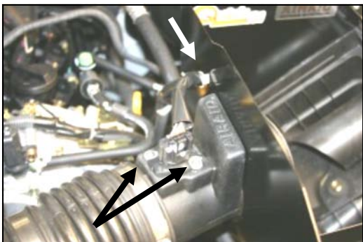
13. Install the MAF sensor from step #5 into the MAF adapter. Use the two supplied button head bolts (#8), to securely fasten the MAF. Do Not Use The Factory Screws! Next push and snap the wire loom retainer from Step #3 into the hole in the MAF panel.
