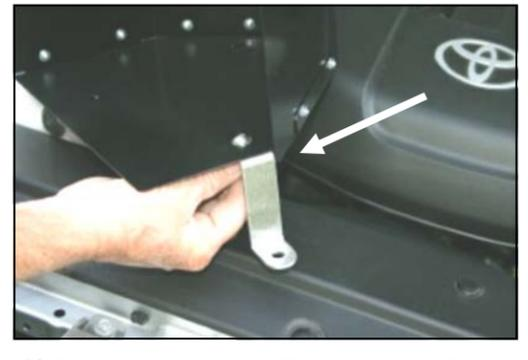
12. Install the bracket (#17) on the front of the CAD using the 1/4-20 button head bolt (#13), 1/4" flat washer (#14), and 1/4" serrated nut (#15), as shown. Just snug the bolt for now, there will be some adjustment needed once the CAD has been installed.
