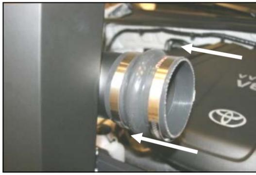
11. Install the urethane hump hose (#4), and two #64 hose clamps (#8) on the tube of the CAD as close to the panel as possible. Leave the hose clamps loose for now.
