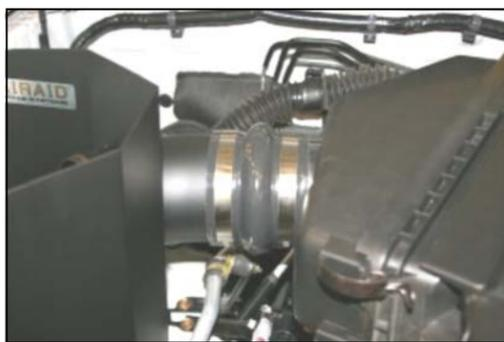
14. Center the hump hose between the tube on the factory airbox, and the tube on the CAD, adjust for fit, and tighten the hose clamps. Now tighten the button head bolt that holds the bracket to the CAD.
