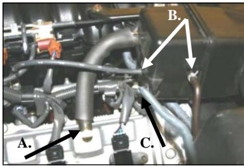
**2.** A) Disconnect the breather hose at the valve cover. B) Disconnect the 1/8" and 1/4" vacuum lines on the back of the factory intake tube. C) Unclip the wiring harness retainer from the back of the intake tube.
