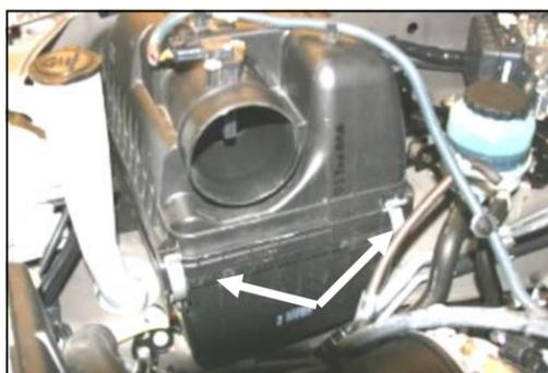
**5.** Unlatch the 4 clips on the factory airbox, and remove the lid.
