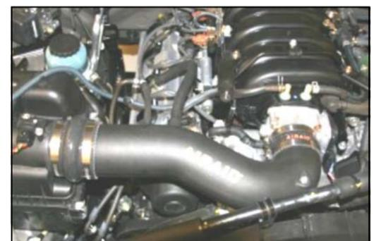
**9.** Install the MIT into the hump hose first, and then into the reducing coupler. Adjust the MIT snugly against the throttle body, and tighten the 4 hose clamps. Next install the 1/4 - 20 x 1/2" button head bolt (#10) and 1/4" flat washer (#11) thru the Adel clamp and into the MIT to hold the air conditioning hose.
