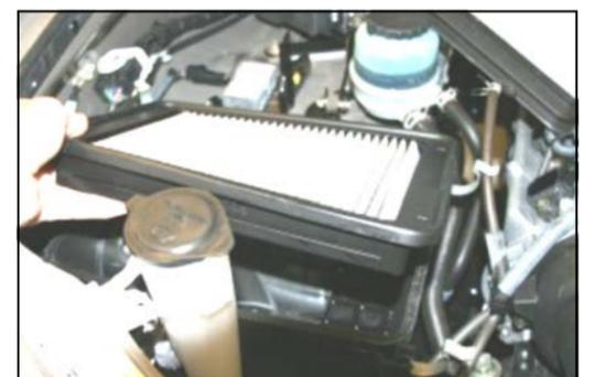
**6.** Remove the factory air filter, and install the Airaid Premium Filter (#1). Reinstall the factory airbox lid, and relatch the 4 clips.
