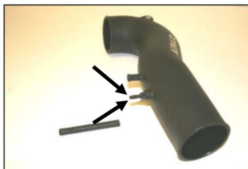
**8.** Install the 1/4" barb x 1/8" NPT fitting (#8) into the Airaid Modular Intake Tube (MIT) (#2) as shown. Now slide the 1/4" x 4" hose (#9) onto the barb fitting.
