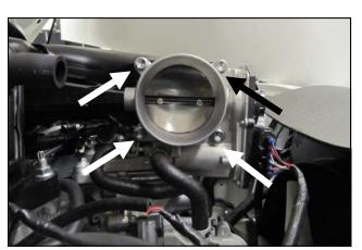
**5.** Install the provided bolts and washers thru the throttlebody and Poweraid Spacer and tighten to the manufacturer's specifications in an X Pattern.
