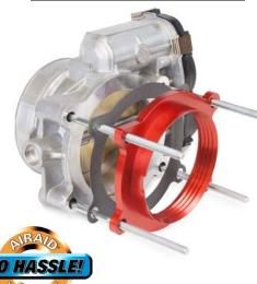
Example of proper spacer installation.
