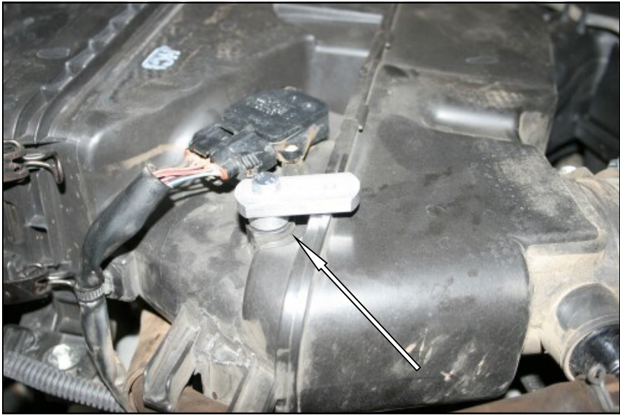
8. Reinstall the resonator/airbox assembly in the reverse order that you removed it using the factory bolts. Make sure to reconnect all breather and vacuum hoses, and the Mass Air sensor electrical connector. Install one 1” extension plate (#9) using the 5/16” thick round spacer (#10) and 6mm x 25mm bolt (#6), with flat washer (#4) in the threaded hole where the stud was removed on the resonator/airbox, with the extension plate facing the throttlebody as shown.
