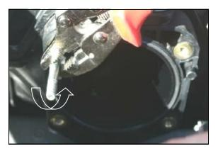
**4.** Using a stud remover or pair of pliers, carefully remove the factory stud from the intake manifold.
