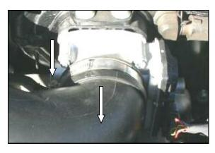
**2.** Using a 10mm socket, loosen the hose clamp on the throttle body end of the intake tube. Slide the intake tube off of the throttle body towards the radiator.
