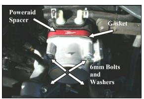
**5.** Position the Poweraid Spacer (#1) and gasket (#2) between the throttle body and intake manifold. Insert four 6mm x 65mm hex bolts (#3), and 6mm flat washers (#4) thru the throttle body, gasket, Poweraid Spacer, and into the intake manifold. Using a 10mm socket, tighten all four throttle body bolts evenly, to the manufacturers specifications.
