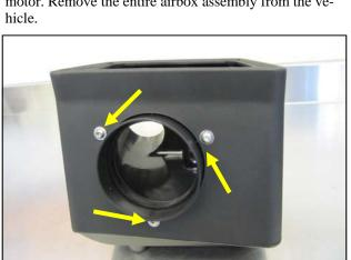
**7.** Mount the Filter Adapter (#5) to the Cold Air Box, as shown, using three 1/4-20 x 1/2" Button head Bolts (#16) and 1/4" Flat Washers (#17).
