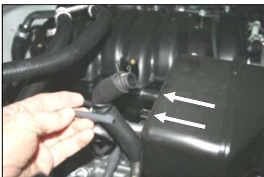
4. Disconnect the breather hose from the back of the factory intake tube and the valve cover. Disconnect the 1/8" vacuum hose from the back of the factory intake tube and the vacuum connection on the engine. These hoses will be replaced with Airaid hoses later in the install.
