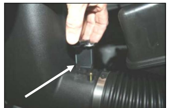
9. Remove two Phillips head screws and remove the MAF sensor from the factory intake tube. It will be reinstalled in step #10.
