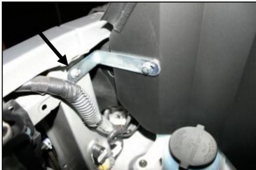
13. Fasten the #203 bracket (#26) to the existing hole in the radiator support using one 1/4-20x1/2" button head bolt (#13) washer (#14), and serrated nut (#15). Tighten all nuts and bolts that hold the CAD to the vehicle at this time.
