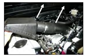
**3.** Unlatch the four metal clips that hold the airbox lid to the base and remove the intake tube and lid from the vehicle. Remove the factory air filter from the airbox base.
