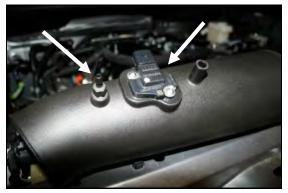
9. Re-install the MAF sensor into the Airaid intake tube (#2) as shown <u>using the supplied 8-32x3/8" button head screws (#12).</u>
