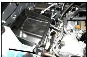
**4.** Using a 10mm socket, loosen the two bolts that hold the airbox base to the fender well, and remove it from the vehicle. There is one bolt on the front of the base, and one bolt at the rear of the base.
