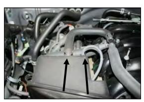
**2.** Disconnect the factory breather hose, and vacuum hose from the factory airbox lid.
