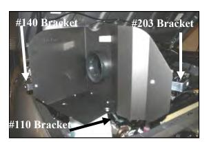
**6.** Assemble the Cool Air Dam panels (#3 & #4) as shown using four 6-32 screws (#9), washers (#10), and keps nuts (#11). Install the filter adapter (#5) using three 1/4" button head bolts (#13) and washers (#14). Install the 3 brackets (#24), (#25), and (#26) as shown using three 1/4" bolts (#13), washers (#14), and nuts (#15). Just snug the bolts for now, they will be adjusted later.
