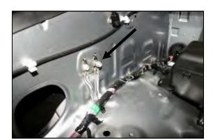
**5.** Remove the rear ground anchor bolt from the side of the fender well and save it for reuse in step #7.
