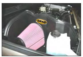
16. Install the Airaid Premium Filter (#1) onto the filter adapter and tighten the clamp. Next install the weather strip (#8) on top of the **CAD** as shown. For an easier install, start at the fender side of the **CAD** and work your way towards the radiator. Reinstall the factory beauty cover. Apply the Airaid Decal to the Panel assembly a shown.
