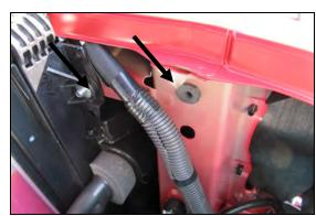
**14.** Place Well Nut into 3/8" hole in core support.
