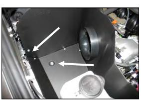
7. Install the **CAD** assembly into the vehicle. Align the hole in the bottom over the captured nut in the fender well. Install one 16mm hex bolt (#16), and washer (#14). Leave loose for now. Next reinstall the factory bolt removed in step #5, thru the bracket, into the ground anchor in the fender well.
