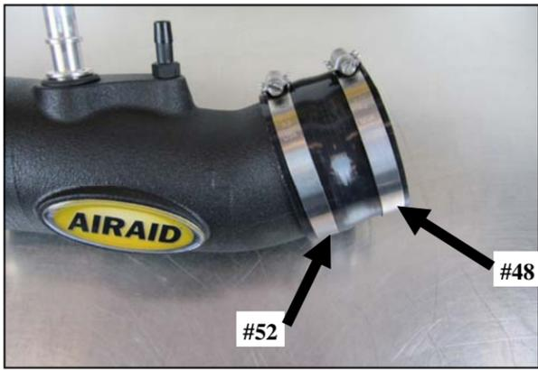
7. Slide the Reducer, one #48 Clamp, and one #52 Clamp onto the other side of the Intake Tube as shown. Do not tighten the Clamps at this time.
