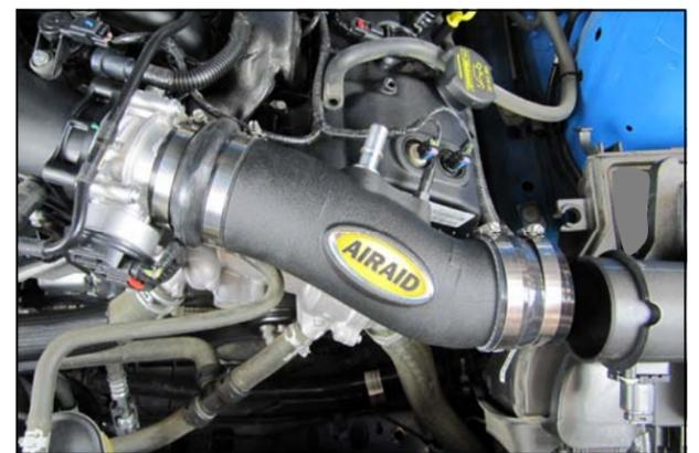
9. Slide the Tube assembly onto the throttle body.
