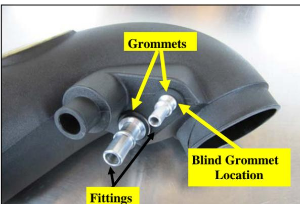
7. Insert the Grommets and Aluminum Fittings into the Airaid Intake tube as shown. On vehicles not equipped with the small breather, plug the hole with the Blind Grommet.
