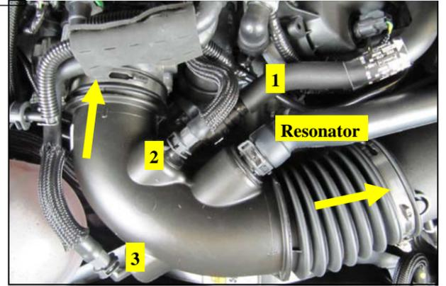
3. Disconnect the 3 breather lines and resonator tube from the intake tube. Loosen the hose clamps and remove the factory intake tube. Depending on your configuration, you may have two or three lines. Loosen the hose clamps and remove the factory intake tube.
