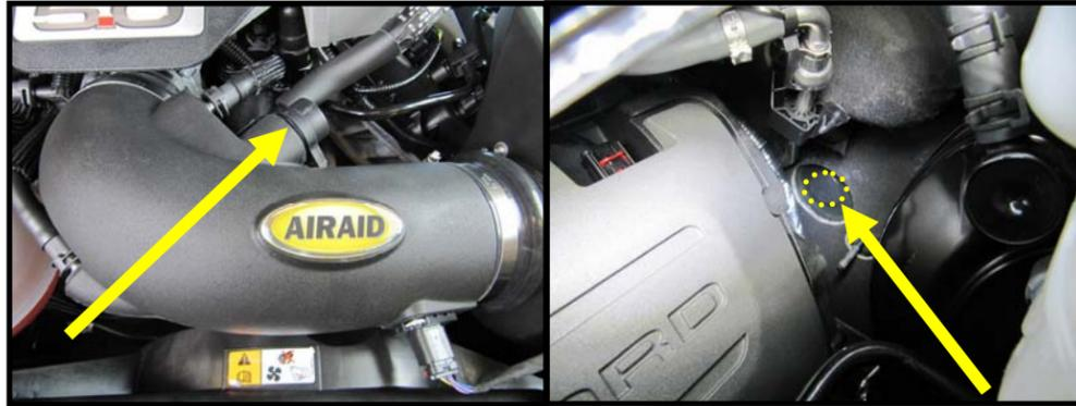
**Resonator Delete Option:** The resonator can be safely deleted if so desired by capping off the Intake Tube with the supplied Cap and Speed clamp. After removing the resonator assembly from the firewall, insert the included Firewall plug to prevent debris from entering the cabin.
