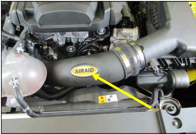
10. Insert the large end of the Intake Tube into the Hu Apply the Airaid Bubble Decal onto the Intake Tube as shown.
