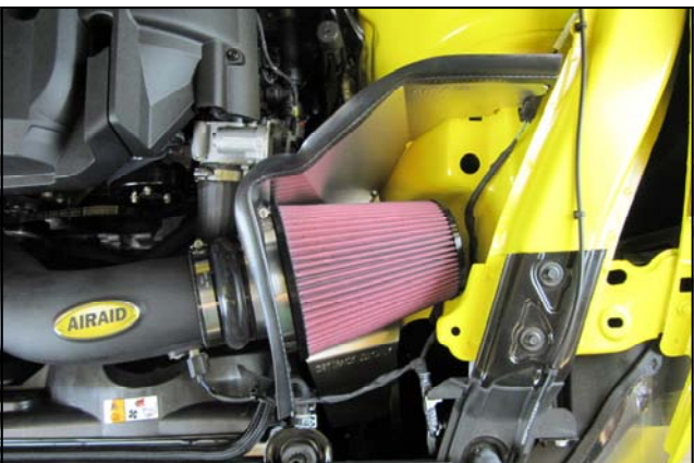
23. Install the Airaid Premium Filter onto the Filter Adapter. Install the weatherstrip on top of the Panel assembly as shown with the contour rolling away from the filter.
