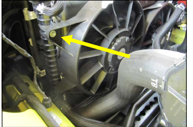
15. Remove the drivers side fan shroud bolt and set it aside.
