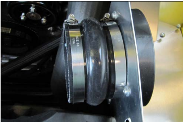
20. Slide the Hump Hose with two, #68 Clamps onto the Filter Adapter .
