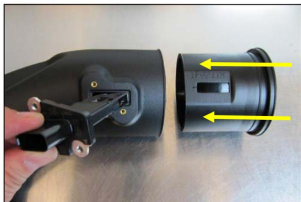
5. Using the supplied Torx driver, remove the MAF sensor from the factory airbox and create the Tube assembly.
