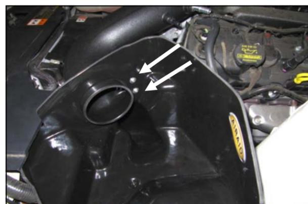
**9.** Secure the Intake Tube to the CAB using the two 1/4" Button Head Bolts (#6) and 1/4" Washers (#7).
