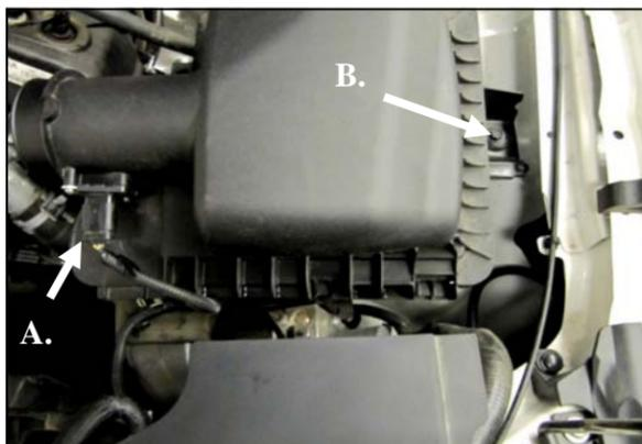
**2.** **A)** Slide the red lock tab back, and disconnect the wiring harness from the Mass Air Flow sensor (MAF). Carefully pry the harness anchor from the air box using a screwdriver. **B)** Using a 10mm socket, remove the bolt securing the air box to the inner fender and remove the air box assembly. This bolt will be reused in step 4.
