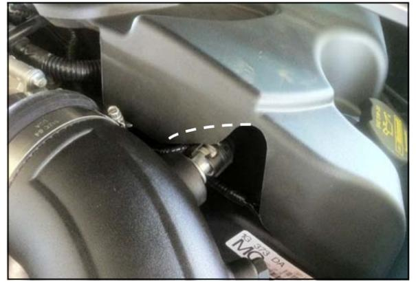
For Performance Package equipped motors, it is recommended that the installer enlarge the breather cut out in the engine cover using a Dremel with a cut off wheel, then de burr for a professional look.
