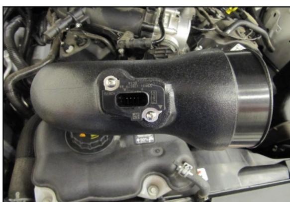
**5.** Transfer the MAF sensor into the Airaid Intake Tube (#2) and secure using the supplied 8-32 Button Head Screws (#8).
