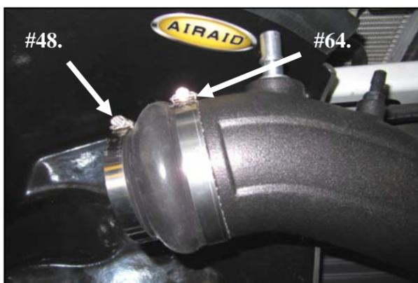
**7.** Slip the Hump Hose (#4) and Hose clamps onto the Airaid Intake Tube. Slide the #64 Hose Clamp (#10) onto the tube side and the #48 Hose Clamp (#9) onto the Engine side. Leave the Hose Clamps loose for now.
