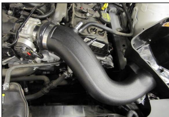
**8.** Insert the Intake Tube into the CAB first, then lower the Tube down and onto the throttlebody. Tighten the Hose Clamps.
