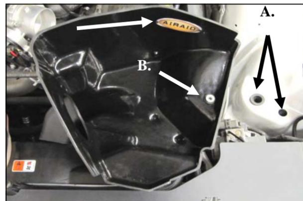
**3.** Transfer the factory air box mounting grommets. **A)** Locate and remove the two lower air box mounting grommets, and install them in the inner fender. **B)** Remove the Upper air box mounting grommet and steel sleeve, and re-install into the Airaid Cold Air Box, or CAB (#3). Apply the Airaid Decal inside of the CAB as shown.
