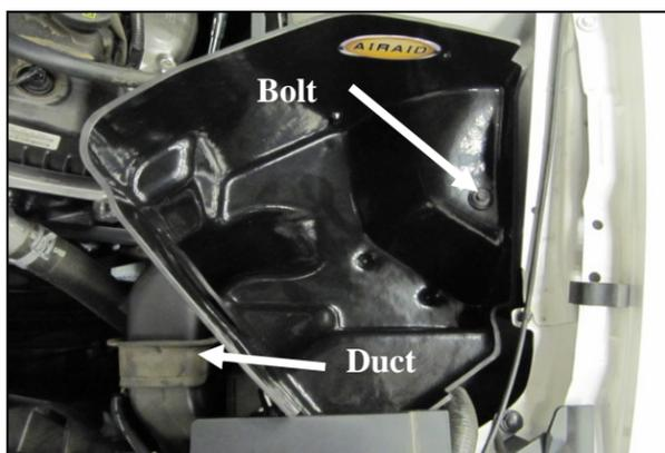
**4.** Install the CAB into the vehicle. Make sure that the Air inlet of the CAB mates with the factory duct, and the two locating cones on the bottom mate with the factory grommets. Next reinstall the factory bolt that was removed in step #3 through the steel sleeve and grommet and into the inner fender.
