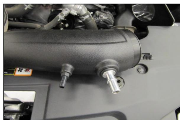
**6.** Install the Grommet and Fittings into the Airaid intake tube. **A)** All models will require the use of the 5/8" Fitting (#11) and the 5/8" Grommet (#12). **B)** Automatic transmission equipped vehicles will also use the 1/4" Barbed Fitting (#14). Manual transmission vehicles will not need the 1/4" Hose Fitting and will use the 1/4" Plug (#13).
