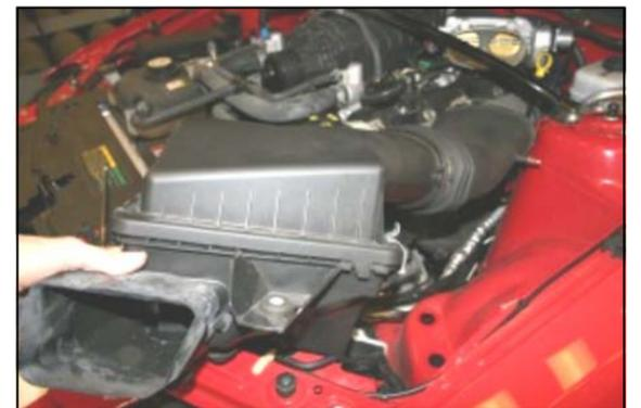
3. Remove the complete factory intake system from the vehicle.
