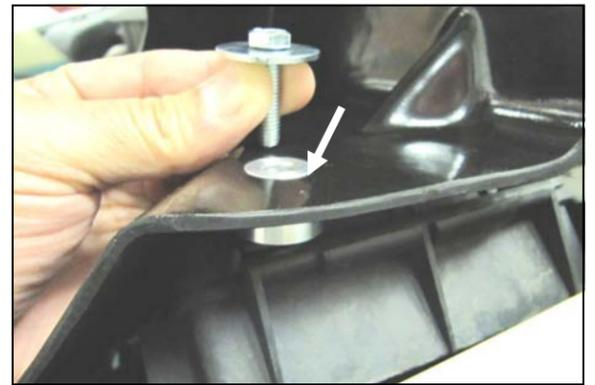
**12.** Slide the Aluminum Spacer (#12) underneath the CAD and into the hole as shown. Secure the CAD to the inner fender using the OEM bolt from step #1 and the supplied 1/4" Fender Washer (#10).
