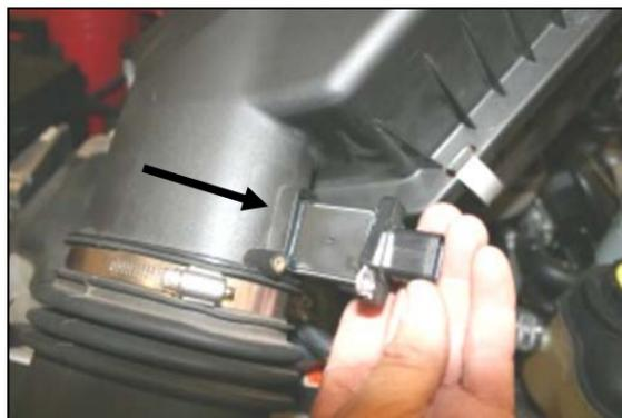
5. Using the provided #20 torx bit, remove two factory screws and the Mass Air Flow sensor from the factory airbox lid. Note the direction of the sensor for proper re-installation later. (Save the mass air sensor for re-installation in step #9, the factory screws will not be re-used).
