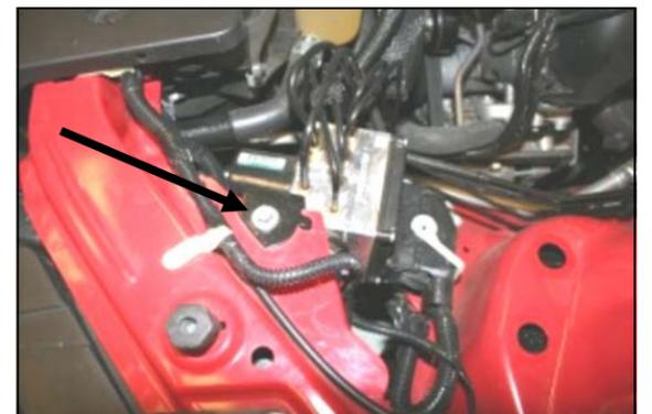
6. Using a 10mm socket, remove and save the bolt from the top of the anti-lock brake bracket. It will be re-installed later in step #13.
