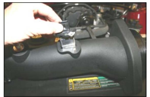
9. Install the Mass Air Flow sensor removed in step #5, into the Airaid Intake Tube **using the provided 8-32 x 3/8" button head screws (#8)**. Make sure the arrow on the sensor is pointing towards the throttle-body.
