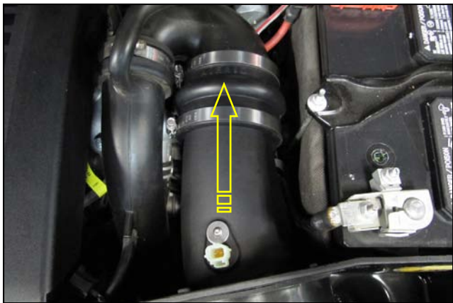
12. Slide the coupler and clamps onto 90 deg. Elbow pipe and tighten the clamps.
