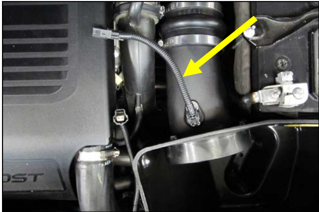
13. Connect the Wire Harness Extension to the air temperature sensor.
