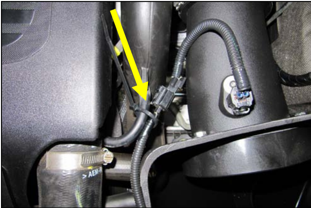
14. Plug the Harness Extension into the factory wire harness and secure it using the supplied Zip Tie. Trim the excess length
