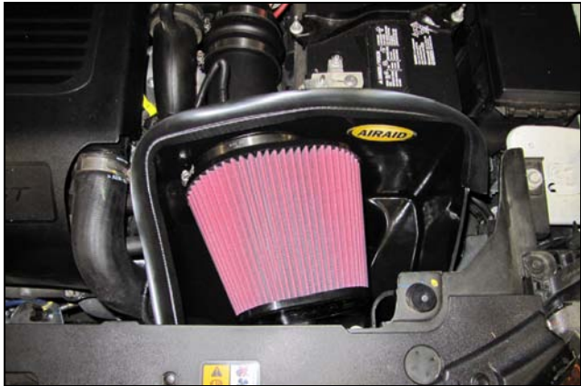
15. Install the Airaid Premium filter onto the Filter Adapter and tighten the clamp. Install the weather strip onto the top of the Air box as shown, with the contour rolling away from the filter.
