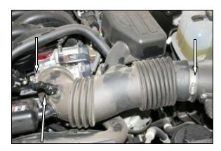
**4.** Re-install the factory intake tube onto the throttle body and the airbox lid, and tighten the hose clamps. Re-connect the breather hose to the factory intake tube.
