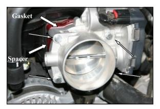
**3.** Insert the four 6mm x 75mm bolts (#3) with washers (#4) thru the throttlebody, one gasket (#2), and thru the Poweraid Spacer (#1), and into the intake manifold. Tighten all four throttle body bolts evenly, to the manufacturer's specifications. **Do Not Over Tighten The Bolts!**
