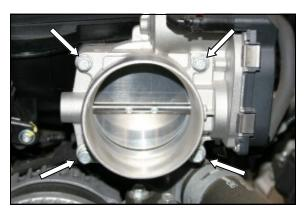
2. Remove the four bolts from the throttle body, and remove the throttle body from the intake manifold, and set it aside. There's no need to disconnect the wiring harness.
