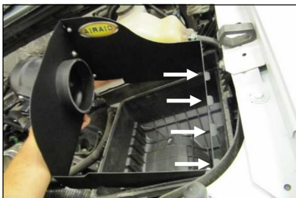
**8.** Install the assembly onto the lower half of the factory airbox. Slide the metal tabs into the airbox slots, and fasten the 3 airbox clips
