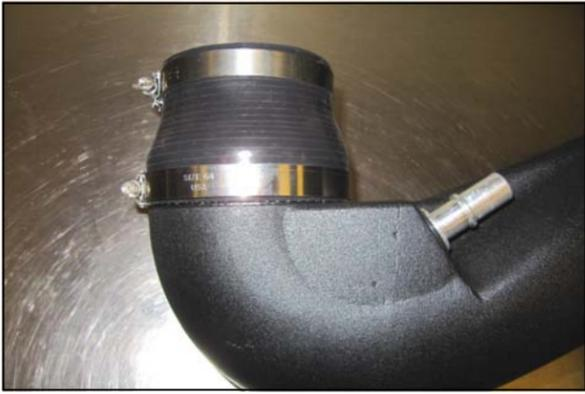
11. Install the Silicone Reducer and Hose clamps onto the Airaid Intake Tube. Place the #56 clamp on the Throttle body side of the reducer, and the #64 clamp on to the tube side.
