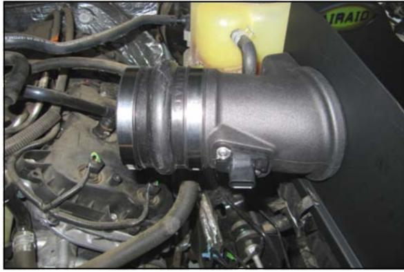
12. Install the hump hose and two hose clamps onto the filter Air Meter Tube as shown. Leave the two hose clamps loose for now
