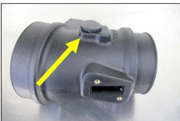
**5.** Insert the MAP Plug into the Intake tube as shown. Hint: Soapy water makes for a good lubricant when inserting the Plug.
