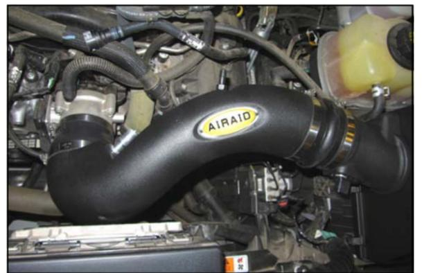
13. Install the Intake Tube onto the throttle body first, then into the Hump Hose. Tighten all of the hose clamps.
