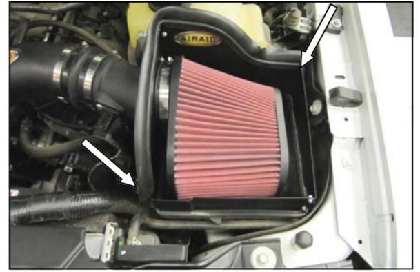
16. Install the Weather Strip onto the panel assembly with the contoured edge rolling away from the filter area. Start at the front of the vehicle and work your way back. Complete the installation by sliding the Airaid Premium Filter onto the Air Meter Tube and tightening the clamp.
