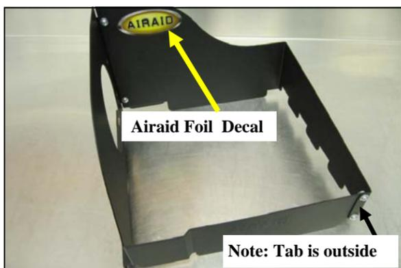
**4.** Assemble the two Quick Fit Panels (#4 & #5) as shown using four 6-32 screws, flat washers, and Kep Nuts. The panel tabs are to be on the outside of the assembly.
