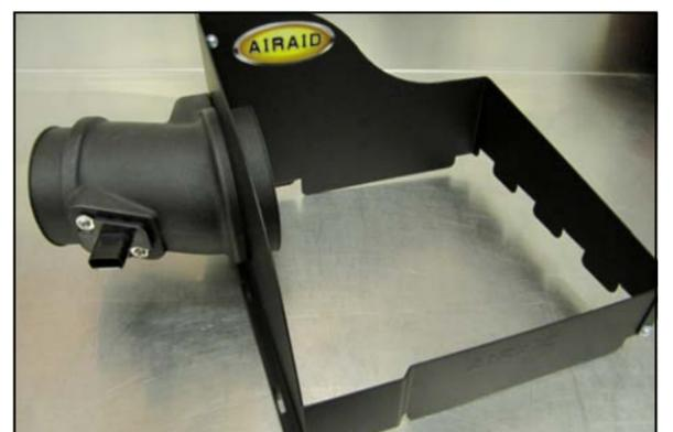
**6.** Transfer the MAF sensor into the Airaid Intake Tube and secure using two 8-32 x 1/2" button head screws. **Do Not Use The Factory Torx Head Screws.**
