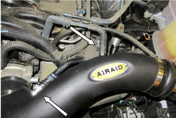
14. Reconnect the breather lines to the Airaid Intake Tube.
