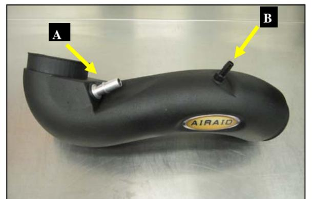
**9. A.)** Insert the 5/8" Grommet into the Intake tube as shown. Complete the tube assembly by inserting the 5/8 PCV Fitting into the Grommet.
