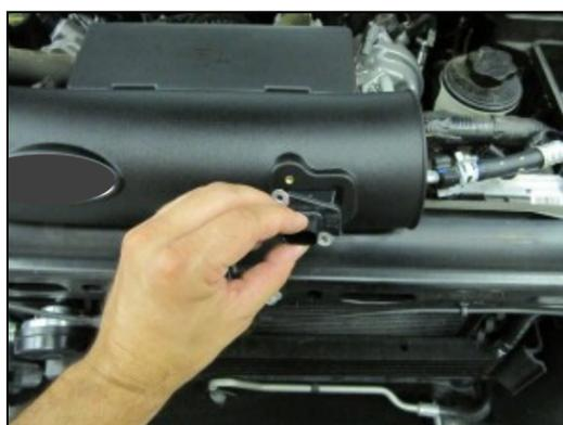
**7.** Transfer the MAF sensor into the Airaid Intake Tube (#2) and secure using two 8-32 x 3/8" button head screws (#11). **Do Not Use The Factory Torx Head Screws!**
