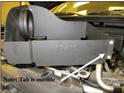
**4.** Assemble the two Quick Fit panels (#3 & #4) as shown using four 6-32 screws (#9) flat washers (#11) and keps nuts (#10).
