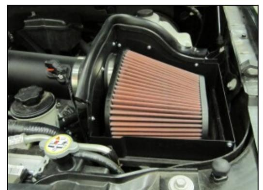
**9.** Install the Airaid Premium Filter (#1) to the mounting flange inside the quick fit assembly. Complete the installation by attaching the Weather Strip (#5) to the top of the panels as shown.
