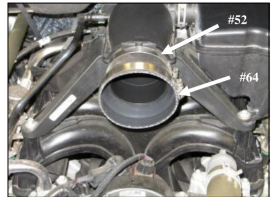
**6.** Install the Silicone Coupler (#6), one #64 Hose Clamp(#14), and the #52 Hose clamp (#13) onto the engine air inlet. Leave the clamps loose for now.
