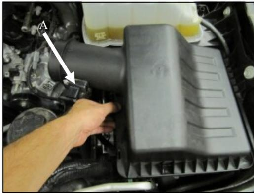
**2. A.)** Disconnect the Mass Air Flow (MAF) Sensor.
