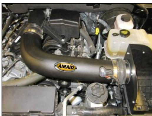
**8. A.)** Insert the Airaid Intake Tube into the couplers as shown. Check for alignment, and tighten all clamps.
