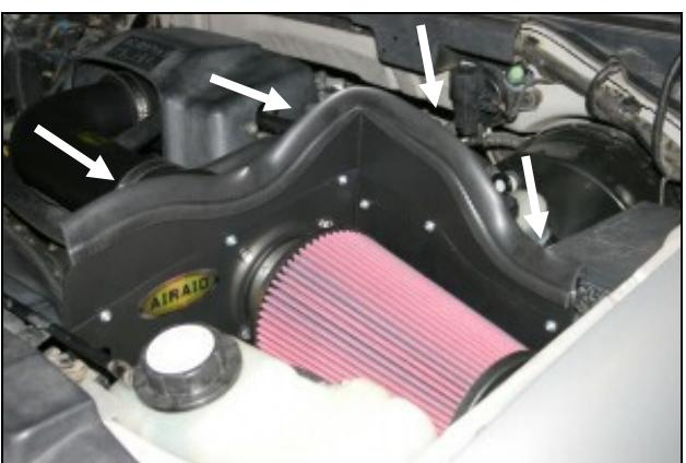
12. If your vehicle **Does Not** have a hood mat, install the panel extension (#4) as shown using five 6-32 Phillips head screws (#5), flat washers (#6), and kep nuts (#7). Next install the weatherstrip (#4) onto the top of the panel assembly as shown.
