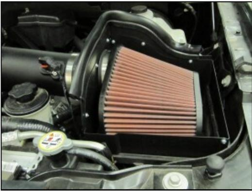
10. Install the Airaid Premium Filter (#1) to the mounting flange inside the quick fit assembly. Complete the installation by attaching the Weather Strip (#5) to the top of the panels as shown.
