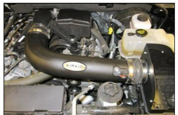
**9. A.)** Insert the Airaid Intake Tube into the couplers as shown. Check for alignment, and tighten all clamps.
