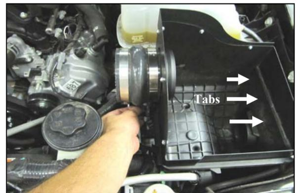
**6. A.)** Install the Silicone Hump Hose (#7) and two #64 Hose Clamps (#14) onto the Quick Fit assembly. Leave the clamps loose for now.
