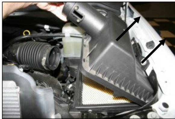
2. Remove the factory airbox lid from the vehicle by sliding the flexible tube off of the airbox lid neck, and then rotate the lid up and out of the base.
