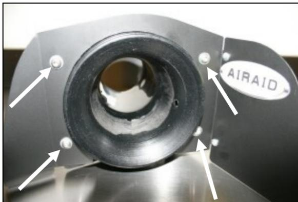
5. Install the MAF Adapter Tube (#2) into the Quick Fit Panel as shown using four 1/4-20 button head bolts (#9) and flat washers (#10). Make sure the slot for the MAF sensor is on the left side when looking from this view.
