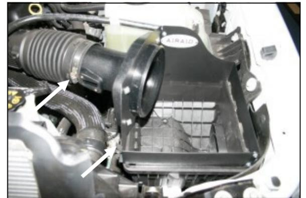
6. Install the Quick Fit Assembly onto the top of the factory airbox base sliding the four tabs on the panel into the slots on the base and then latching the three factory latches. Slide the factory intake tube over the MAF tube and tighten the factory hose clamp as shown.
