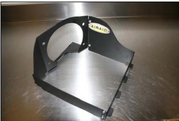
4. Assemble the two Quick Fit panels (#3 & #4) as shown using four 6-32 screws (#6) flat washers (#7) and keps nuts (#8). Apply the Airaid Decal onto the Panel assembly as shown.
